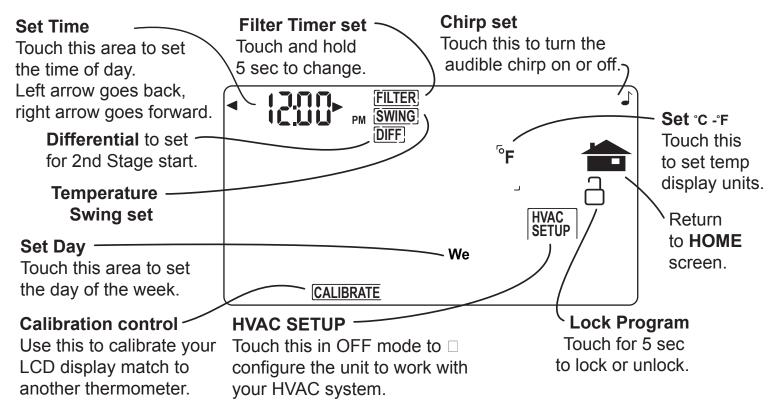
**PROGRAM Screen** The stand alone **PROGRAM** screen sets the CT30 control for your home HVAC system with out a central controller. Press and hold PROG for 10 sec to access it. After that it is displayed when you press the PROG button. [See page 8 for details]
